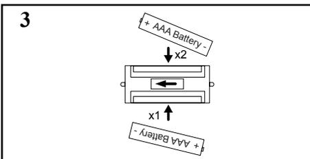
Then insert the batteries into the cage correctly - 2 of the AAA Batteries go in the battery cage one way and the third one goes in the other.
