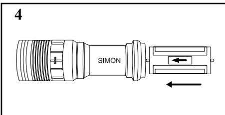
Make sure you place the battery cage in the Flashlight correctly with the 2 positive connections on the batteries pointing towards the front of the flashlight. There should also be a white sticker with RED arrow on the Battery cage, Point that arrow towards the front of the flashlight.
