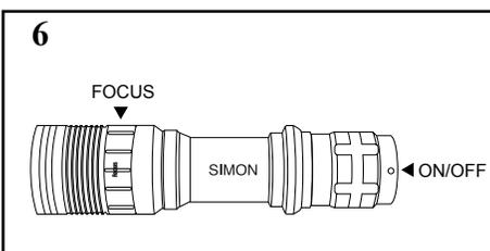
Turn the flashlight On/Off by Pressing the Rear Butt Trigger Switch ALL THE WAY DOWN. After you press the switch and the flashlight is ON you have the option to use other modes the Simon Flashlight has to offer. You just have to soft touch by pressing lightly the trigger switch located at the rear of the flashlight.(AKA on/off button) You will be able to cycle through several modes. Just soft touch into your next mode. High, Medium, Low, Strobe and SOS.
