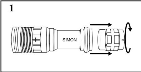
Insert 3 AAA Batteries by unscrewing the rear butt Trigger Switch Cap and removing the battery cage. Make sure that when you place the 3 AAA Batteries that they are fully charged.
