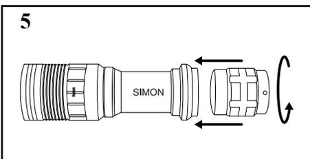
Screw the Rear butt Trigger Switch Cap back on.
