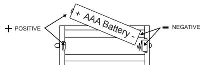
Be sure the Negative side of the battery touches the Spring in the battery cage and the Positive touches the flat Metal Plate on the opposite side.
